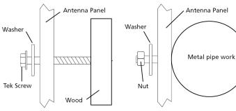
Using the defined mounting holes, mount the Antenna Panel on the outside of the animal handler so that the middle of the Antenna Panel matches the average height.
